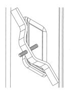
INSERT MOUNTING BRACKET INTO HAND HOLE. WHILE HOLDING COVER PLATE FIRMLY IN PLACE, TIGHTEN BOLT UNTIL COVER PLATE IS SECURE.
